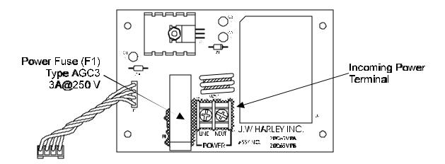
Figure 2-6: Power Supply Circuit Board
